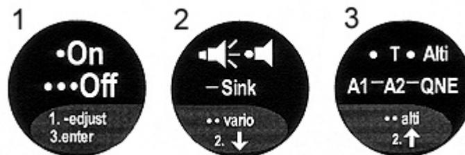
**Log book:** -start the instrument and wait for the control-display. After push key-no. 2 and 3 together- The last flight with flying-time will be shown in the memory (**-0P**)
