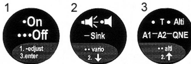
**Start:** -push key-no. 3 and hold and start the instrument on same time. The display shows a (d) or a (b) - (d= hangglider-paraglider-mode, b= ballon-mode)
